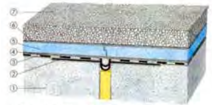
① Decke ② Elastic joint ③ PVC Membrane ④ Non-woven fabric ⑤ Insulation ⑥ Non-woven fabric ⑦ Gravel
