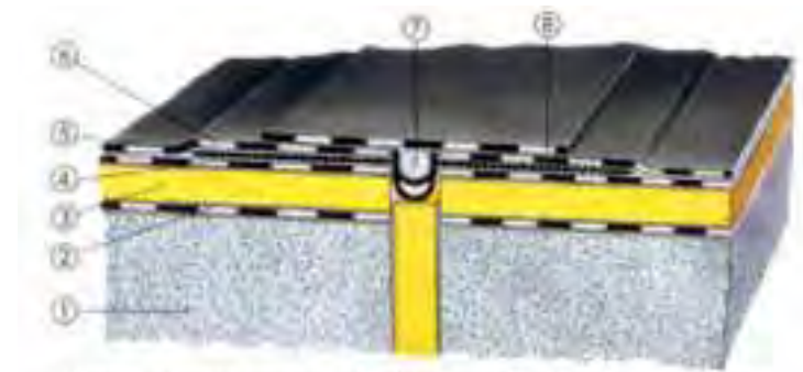
① Decke ② Slabs frame ③ Insulation ④ Membrane ⑤ Elastic joint ⑥ Membrane ⑦ Polyurethane foam filler ⑧ Partially attached membrane
