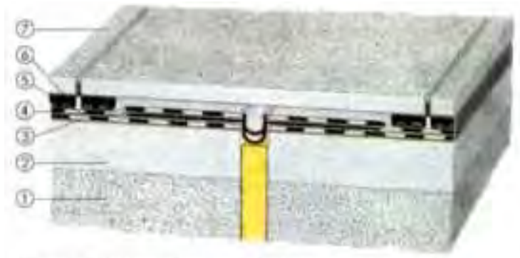
① Decke ② Lightweight concrete ③ Membrane ④ Elastic joint ⑤ Membrane ⑥ RAU-PROFIL support ⑦ Paving slabs
