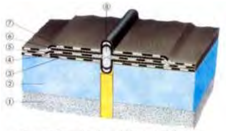
① Decke ② Insulation ③ Membrane ④ Elastic joint ⑤ Membrane ⑥ Double elastic joint ⑦ Membrane ⑧ Double polyurethane foam filler
